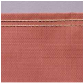
WSC36149 60"X50YDS 15 OZ Fiberglass Blanket Red Approved for use in vertical applications with light-moderate exposures resulting from chipping, grinding, heat treating, sand blasting and light horizontal welding. Prevents sparks from escaping a confined area
