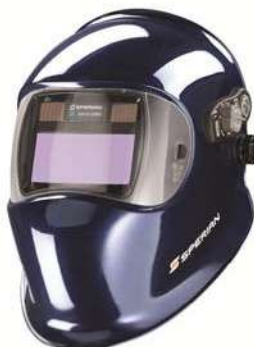
Optrel e680 Welding Helmet, Shade Range 5-13 3-way adjustable headgear. Can be used for overhead welding. Control unit on the outside of the helmet. Grind mode. Sensitivity/Delay functions. Shade range 5-13. True color filter. Variety of adjustable features
