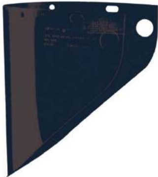
FM4199IRUV5 Faceshield Window Extended View .060" 9 3/4" X 19" IR/UV Shade 5, Injection Molded, Fits F400 and F500 Series and FH66
