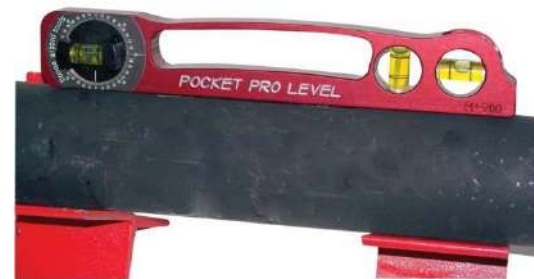
FLAPP-200 Pocket Pro Level 2.5 Increments. Extra strong magnets hold it firmly to any steel surface. Magnetic. There are two (2) stationery vials placed at 90° angles of each other and can be read from any surface of the level. With protractor degree dial
