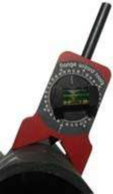
FLA53205 Magnetic small centering head w/vial Designed to establish and mark a centerline at any angle around the circumference (inside or outside) on a pipe or tank. Magnetic. Use it as a protractor level, or remove and use the hardened center punch for other marking jobs
