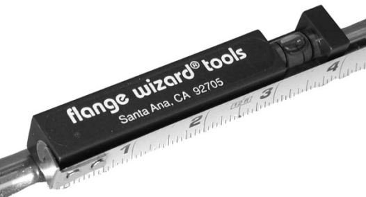
FLA89754 Universal Magnetic Tapeholder A strong 25 pound pull magnet set in epoxy secures the tape holder to your work. It has been redesigned with no removable parts and works with most industrial measuring tapes. It is a great little magnetic pocket level and your third hand when doing those difficult measuring jobs while working alone. Will secure the end of your tape while laying out close tolerance measurements from the end or the center of your material
