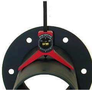
FLA53276 Magnetic Standard Centering Head with Vial Designed to establish and mark a centerline at any angle around the circumference (inside or outside) on a pipe or tank. Magnetic. Use it as a protractor level, or remove and use the hardened center punch for other marking jobs
