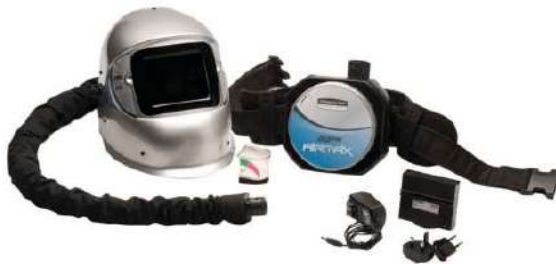
KCP12993 Airmax PAPP with Welding helmet with a W40 Series variable auto-darkening filter which can automatically detect weld arcs and switch to weld shade. Flame-retardant face seal protects against sparks. Lightweight blower unit with adjustable waist belt. Audible alarm signals user when new filter or battery charge is needed. Filter provides NIOSH-approved HE filtration from particulate contaminants
