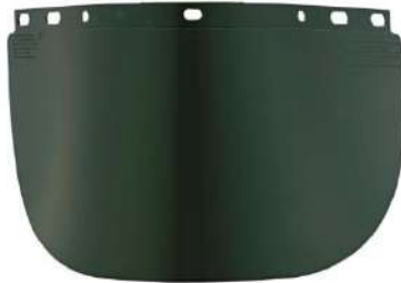
FM4199DGN Faceshield Window Extended View .060" 9 3/4" X 19" Dark Green, Injection Molded, Fits F400 and F500 Series and FH66.
